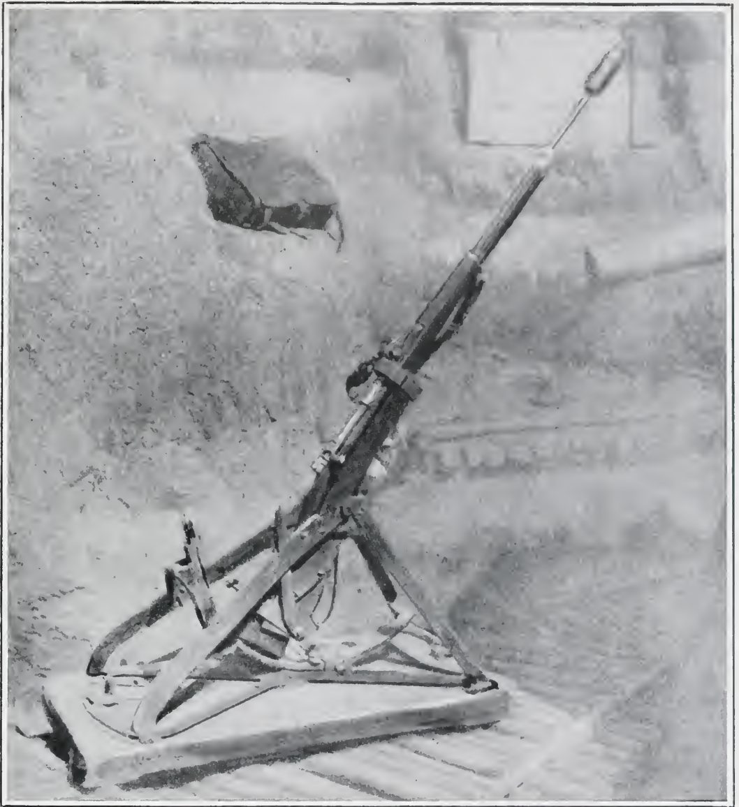
A GERMAN GRENADE-THROWING RIFLE AND ITS SUPPORT.
